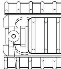
To remove the hand protectors from the RAS, depress the spring lock (2) and slide the top and bottom hand protectors off of the rail. The top hand protector (3) is removed to the rear; the side (4) and bottom (5) hand protectors are removed forward, past the front sight.
